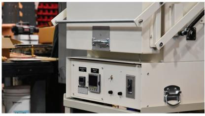
Model GS1714 is as described in Bulletin GS1714-09-14 with angle iron stand. An Industrial Control Option is included consisting of a Eurotherm Nanodac Recorder/Controller and a Eurotherm 3216i overtemperature control. Power control is by solid state contactor.
