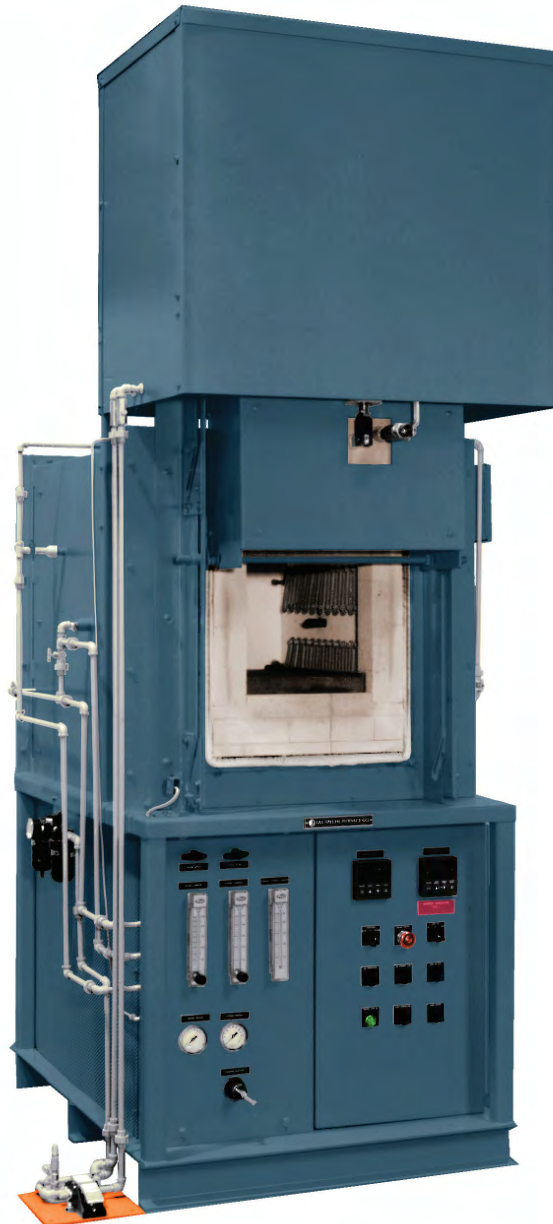
The CBH 124 box furnace is specifically designed for neutral hardening. With the Nitrogen/Propane Atmosphere Package the furnace will do neutral hardening with virtually no decarburization or oxidation
