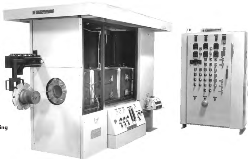
This hydrogen tube furnace is used for processing monochromatic glass. It is uniform to within +/- 2°F.
