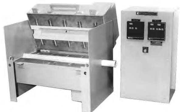
This is a simple TB 224 with a ceramic tube open on both ends.
