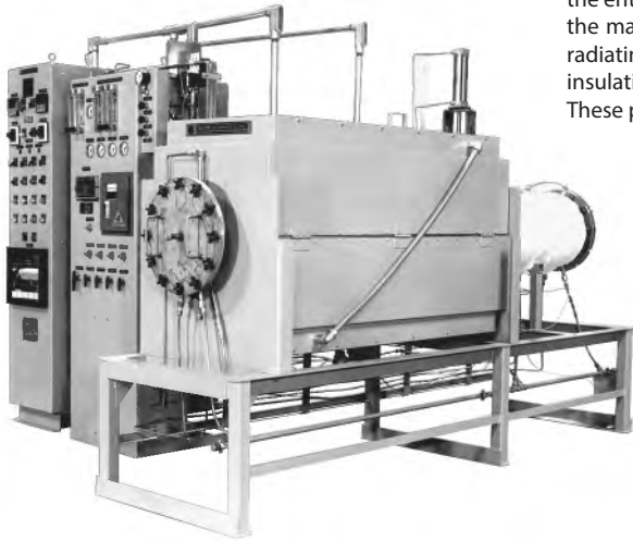
This is a special tube furnace with a hydrogen and oxygen control system and a cooling chamber with a heater. It is used for modeling steel processing cycles.
