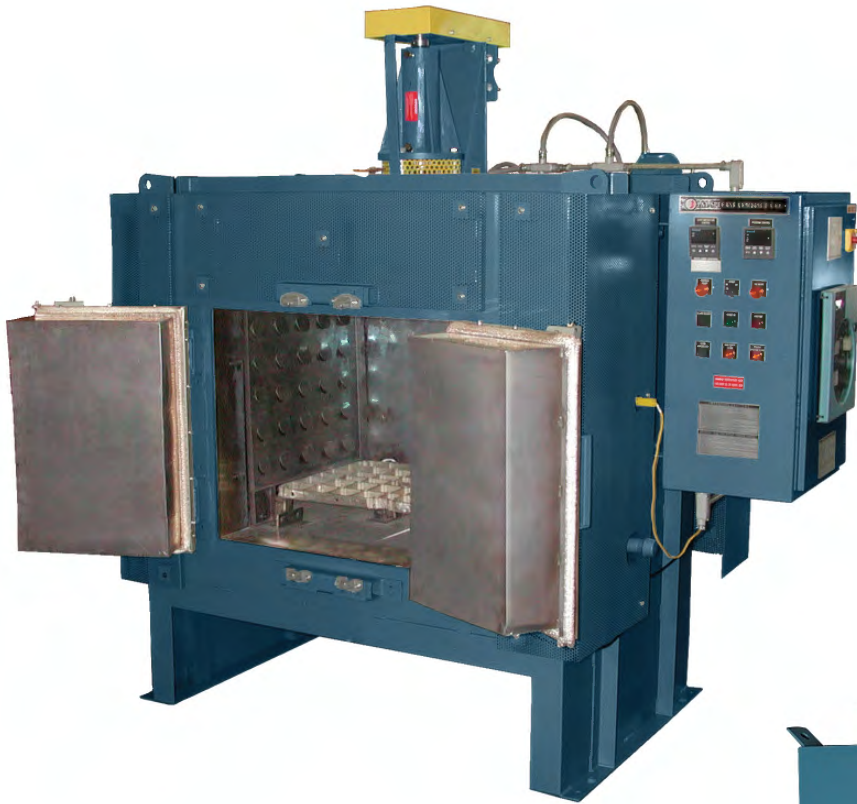
A DV 3648 with double horizontal doors is shown above. DV ovens that are 36" or wider (custom sizes) have double doors like this. Models that are 24" wide have a single door.
