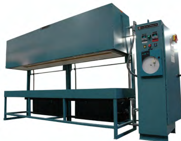
Model WQ8 with NEMA12 panel, program control, overtemp, SCR and chart recorder.
