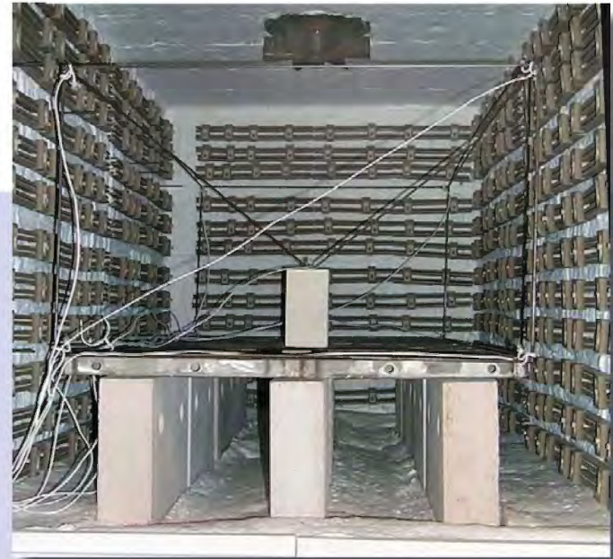
Factory uniformity surveys are routinely done to insure certification upon commissioning
