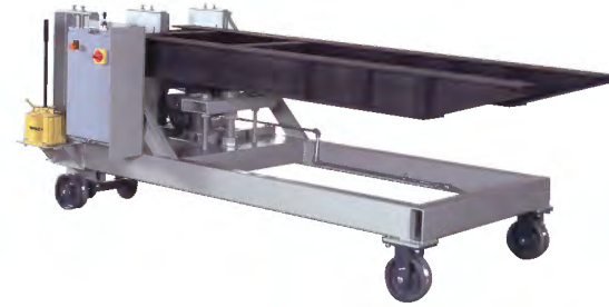
This is a special 2000 pound loader with a motorized mover for heavy loads. It runs on a railroad type track. A deadman joystick control operates the drive system. The handle at the back is the hand pump for the hydraulic lift system
