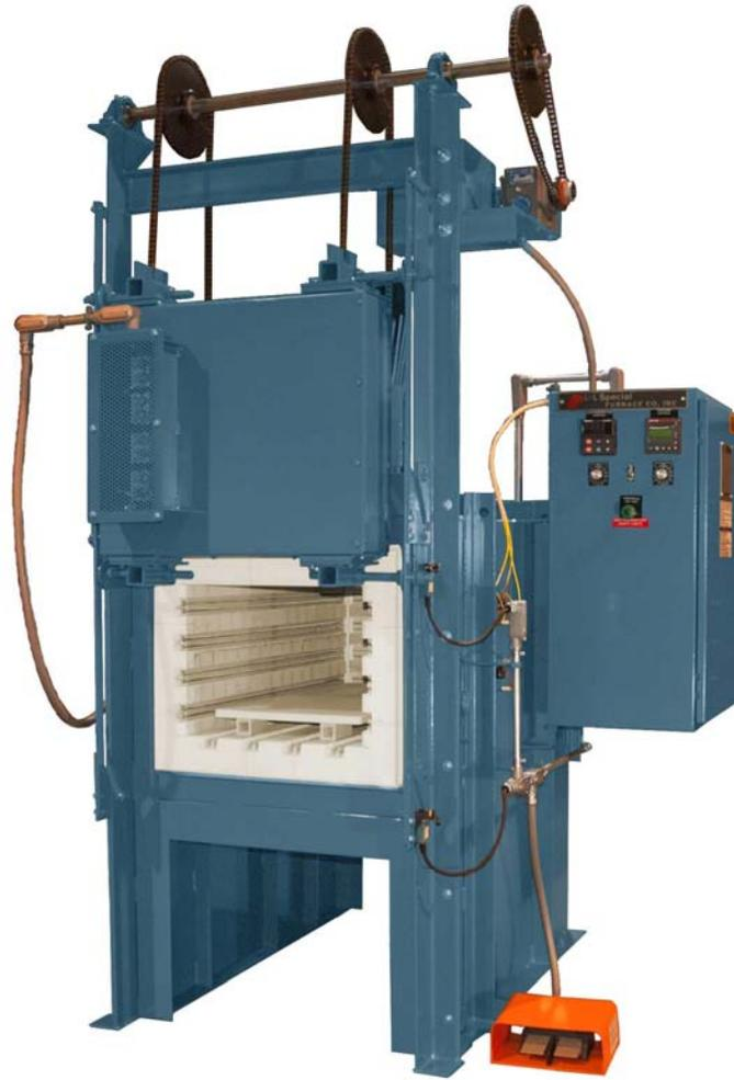
Model XLE814 High Uniformity Floor Standing Furnace for a wide Variety of Thermal Applications and Specifically Designed for Hardening Tool Steels
