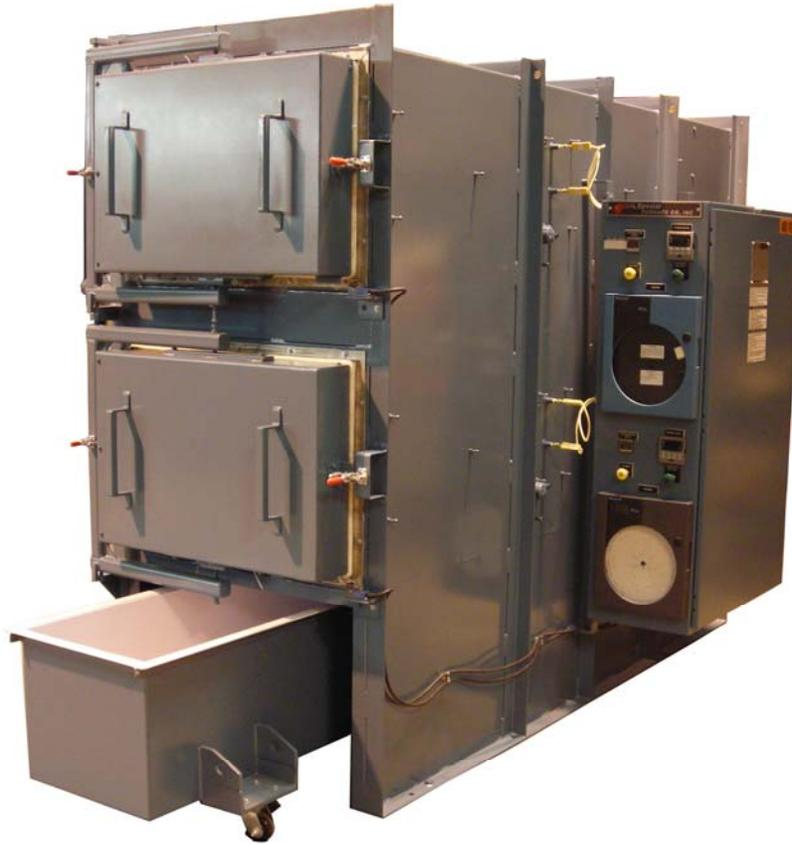
**Model DCA816 Dual Chamber Box Furnace for Heat Treating Aluminum Parts**
