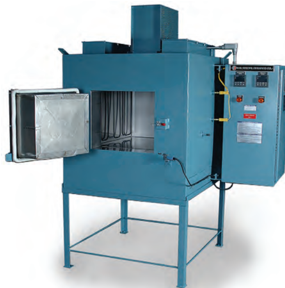
This shows the interior of the VB124. You can see the fan and elements.
